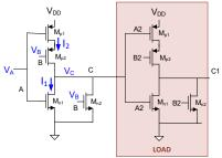
There are two scenarios that cause the output to transition. One is when one of the inputs transitions and the other input is low. The other is when both inputs transition together. We will denote these as Case 1 and Case 2.
