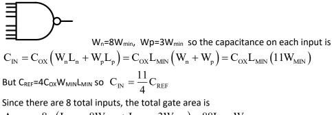
$$A_{GATE} = 8 \bullet \left( L_{MIN} \bullet 8W_{MIN} + L_{MIN} \bullet 3W_{MIN} \right) = 88L_{MIN}W_{MIN}$$
