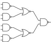
For the inputs on the 2-input NAND gates,  $W_n = 2W_{min}$ ,  $W_p = 3W_{min}$  so the capacitance on each input is  $C_{IN} = C_{OX} \left( W_n L_n + W_p L_p \right) = C_{OX} L_{MIN} \left( W_n + W_p \right) = C_{OX} L_{MIN} \left( 5W_{MIN} \right)$
