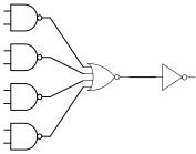
For the inputs on the 2-input NAND gates,  $W_n = 2W_{min}$ ,  $W_p = 3W_{min}$  so the capacitance on each input is  $C_{IN} = C_{OX} (W_n L_n + W_p L_p) = C_{OX} L_{MIN} (W_n + W_p) = C_{OX} L_{MIN} (5W_{MIN})$ But  $C_{REF} = 4C_{OX}W_{MIN}L_{MIN}$  so  $C_{IN} = \frac{5}{4}C_{REF}$  Since there are 8 inputs at the first level of logic, the gate area at the first level of logic is
